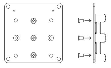
2. Fix the enclosure with the M6 bolts to the plate. Maximum force 6Nm.
